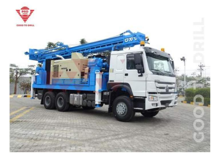
A combination bore hole drilling rig with a pull up force of 18000 kg capable of drilling 6  $\frac{1}{2}$ " diameters up to 600 m depth. Drilling hole size range from 6  $\frac{1}{2}$ " to 14".
