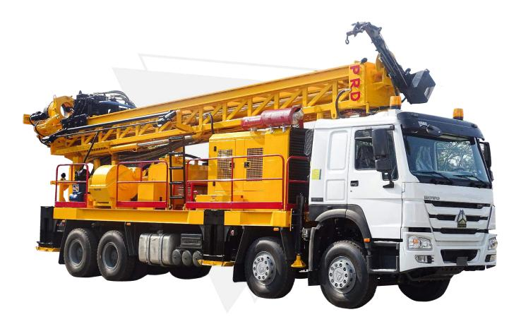
A super performer bore hole drilling rig with a pull up force of 42200 kg capable of drilling 6 ½" diameter up to 1350 m depth. Drilling hole size range from 6 ½" to 20".
